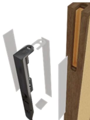
Flush bolt installation and intumescent protection
