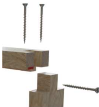
Mortice & Tenon Joint
