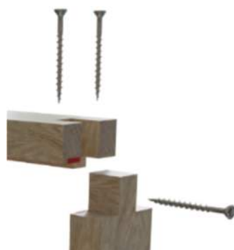
Mortice & Tenon Joint
