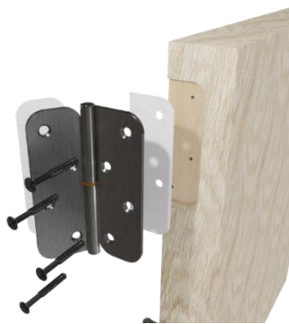
Example of hinge protection detail
